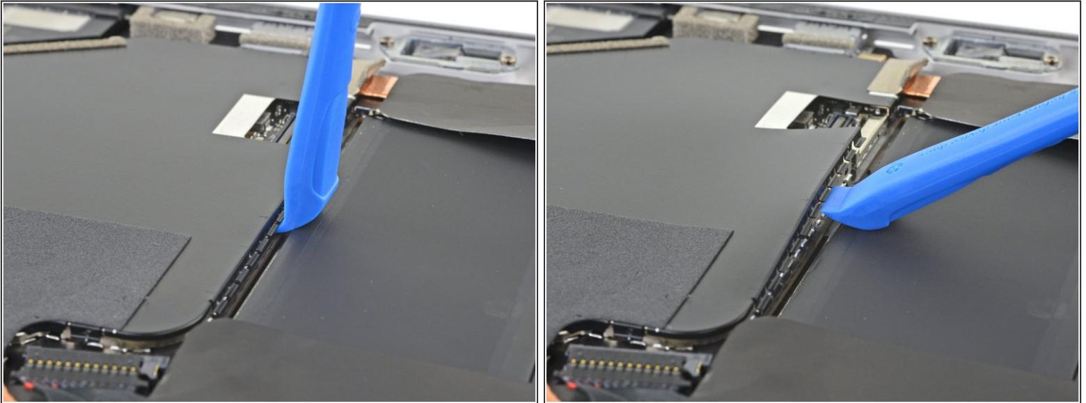
**⚠ Be careful not to puncture or deform the battery with your opening tool.**
