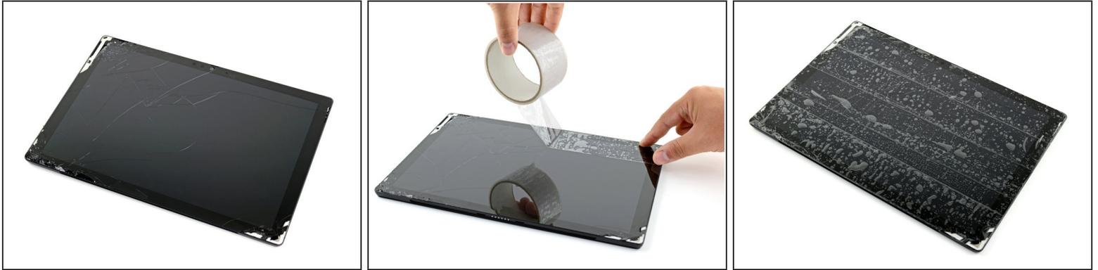
**⚠** Wear safety glasses to protect your eyes, and be careful not to damage the LCD screen.
