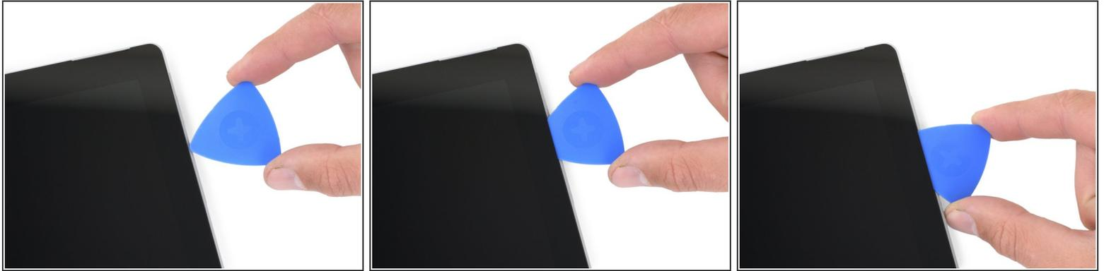
**⚠️ Fragile antenna cables lie under the top edge of the screen. Carefully follow the procedure to avoid damaging them.**
