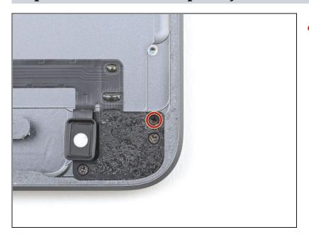
Use a Phillips screwdriver to remove the 2.8 mm-long screw securing the headphone jack to the rear case.
