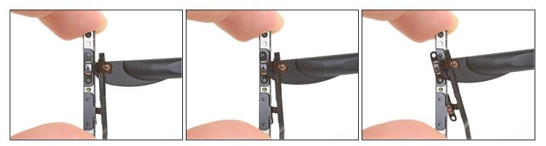
• Insert an opening pick or a halberd spudger underneath the upper volume button to peel it away from the bracket.
