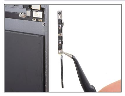
• Remove the volume button bracket from the rear case.
