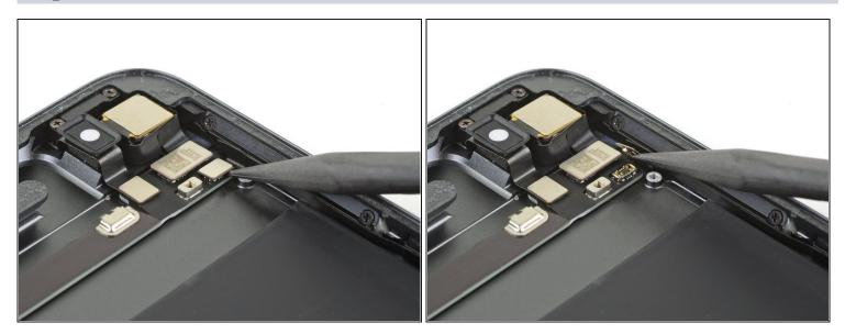
• Use the pointed end of a spudger to disconnect the volume button cable by lifting straight up on the press connector.
