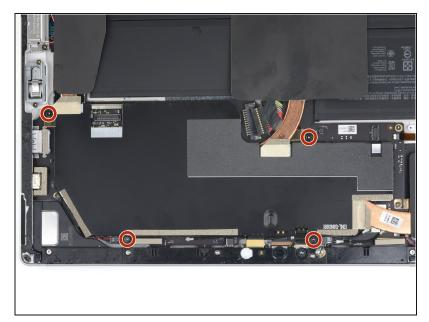
Use a T3 Torx screwdriver to remove the four 2.4 mm screws securing the EMI shield.
