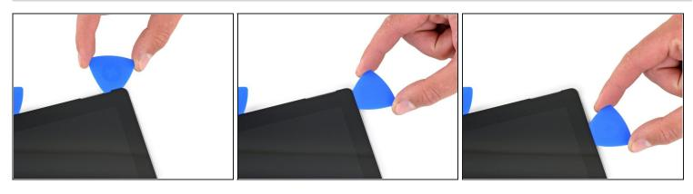
• Round the left corner with the opening pick and slide it along the top edge of the Surface. Stop when the pick is 2.75 inches (70 mm) away from the left edge.
