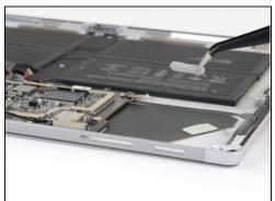
• Push the volume and power buttons into the inside of the case and remove them.
