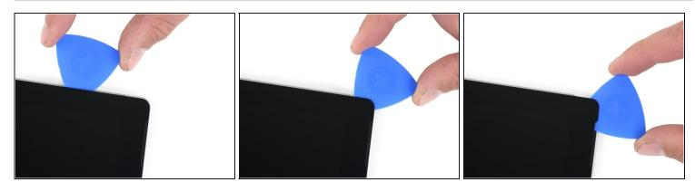
• Once you cut the adhesive over the antennas (8.5 inches, or 22 cm, from the left edge), slide the pick the rest of the way along the top edge of the surface and round the top right corner to slice through any remaining adhesive.
