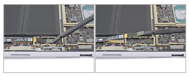
• Use the flat end of a spudger to lift up and disconnect the microSD card reader ribbon cable.
