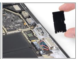
Use an opening tool to pry up on the edge of the EMI shield covering the microSD card reader connector and remove it from the motherboard.
