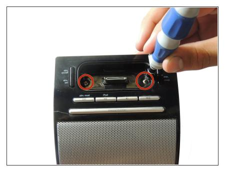
Remove the two 9mm screws that hold on the dock connector with a Phillips #1 Screwdriver.
