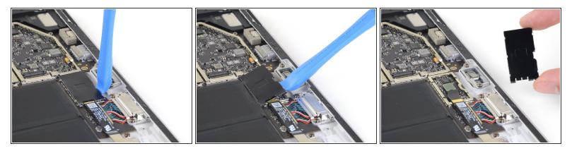
• Use an opening tool to pry up on the edge of the EMI shield covering the microSD card reader connector and remove it from the motherboard.
