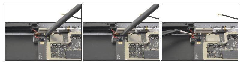
Use the flat end of a spudger to flip up the white plastic locking flap of the ZIF connector at the topleft corner of the motherboard.
