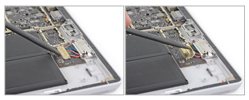
• Use the flat end of a spudger to lift the flap that secures the Surface Connect port connector.
