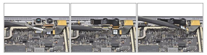
Use the flat end of a spudger to pry up and disconnect all three camera connectors from the motherboard.
