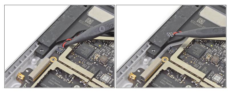
Use the pointed end of a spudger to gently lift the right speaker wire connector straight up and disconnect it from the motherboard.
