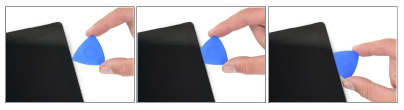
Fragile antenna cables lie under the top edge of the screen. Carefully follow the procedure to avoid damaging them.
