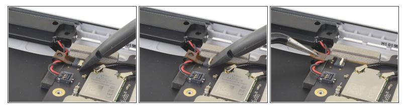
Use the flat end of a spudger to flip up the white plastic locking flap of the ZIF connector at the bottom-left corner of the motherboard.
