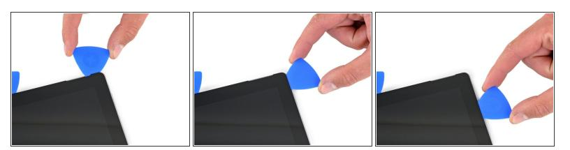
• Round the left corner with the opening pick and slide it along the top edge of the Surface. Stop when the pick is 2.75 inches (70 mm) away from the left edge.
