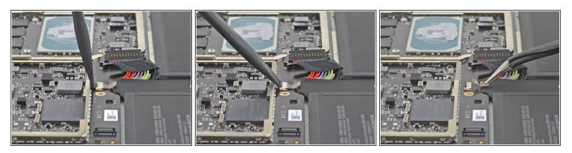
Use the flat end of a spudger to flip up the black plastic locking flap of the ZIF connector at the bottom center of the motherboard.
