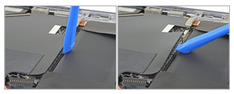
$\bigwedge$  Be careful not to puncture or deform the battery with your opening tool.
