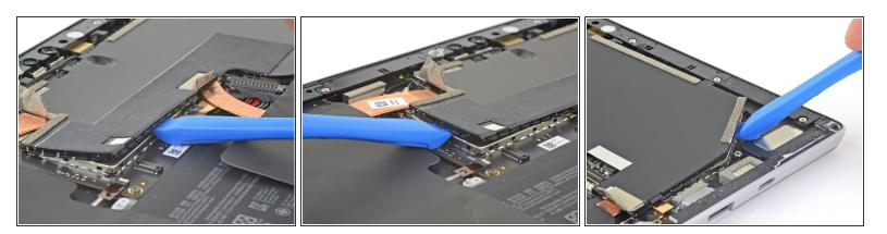
Continue using your opening tool to disconnect the clips around the entire perimeter of the motherboard EMI shield.
