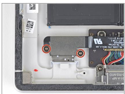
Use a T5 Torx screwdriver to remove the two 3.1 mm screws securing the microSD card reader.
