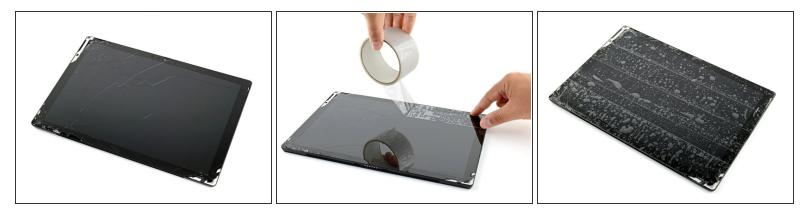
Near safety glasses to protect your eyes, and be careful not to damage the LCD screen.
