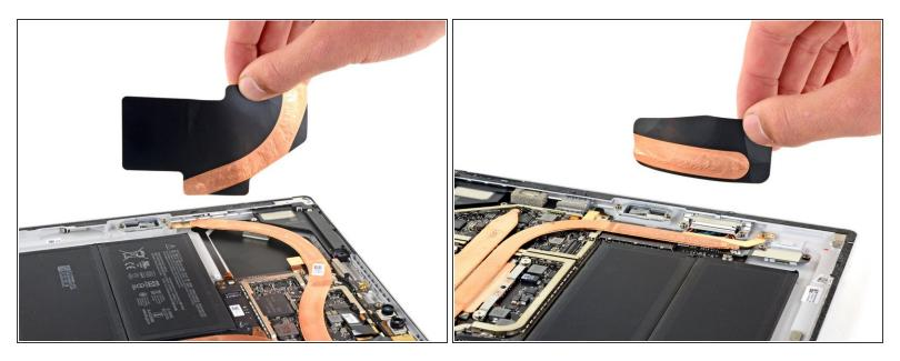
• Peel the remaining two thermal pads off of the heatsink.
