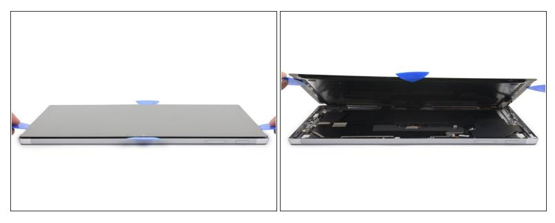
• Very slowly lift the screen assembly away from the Surface case. If you encounter any resistance, stop and check that all the adhesive is separated.
