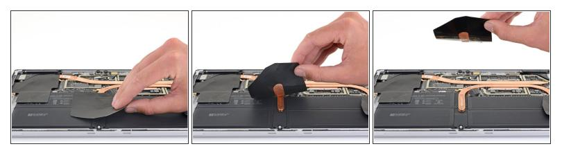
Gently peel the center thermal pad off of the copper heatsink.
