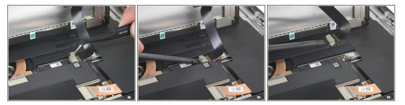
Use a pair of tweezers to peel back the silver tape securing the right display cable to the motherboard.
