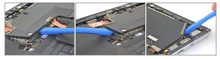
• Continue using your opening tool to disconnect the clips around the entire perimeter of the motherboard EMI shield.
