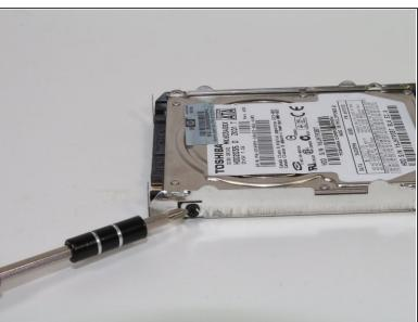
Flip over the hard drive assembly and remove two 4mm Phillips #1 screws at the top left and right side of the hard drive housing.
