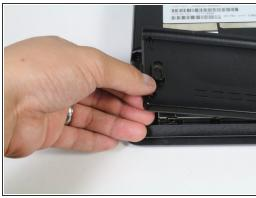
Using a plastic opening tool, open the compartment and remove the compartment cover.
