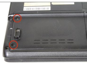
Locate the hard drive in the left hand corner, and remove the two 4mm Phillips #1 screws.
