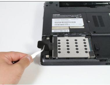
• Use a pair of metal tweezers to grab the plastic pull-tab that is tucked in underneath the hard drive.
