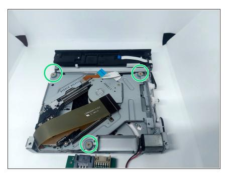
Unscrew the three Phillips #0 screws mounting the optical drive laser.
