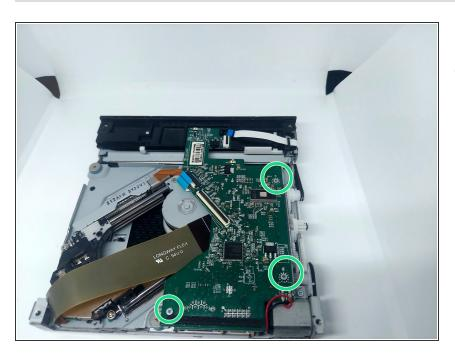
Unscrew the three Phillips #0 screws mounting the PCB.
