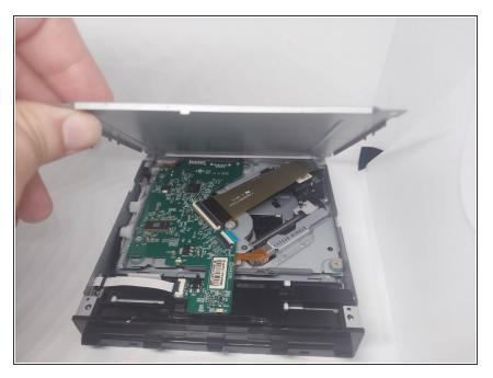
Lift the lid off of the optical drive case, this should require little to no force.
