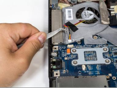
Using tweezers, disconnect power cable by gently pulling white end straight away from its socket.
