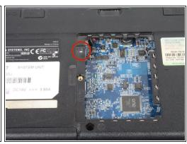
Remove one 1.5mm Phillips #1 screw located near the top left edge of the opening.
