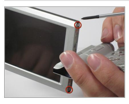
Remove the two 1.5mm screws on the bottom of the screen module with a Phillips #00 screwdriver.
