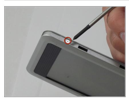
Remove four 2.0mm screws on the side of the screen portion of the device with a Phillips #00 screwdriver.
