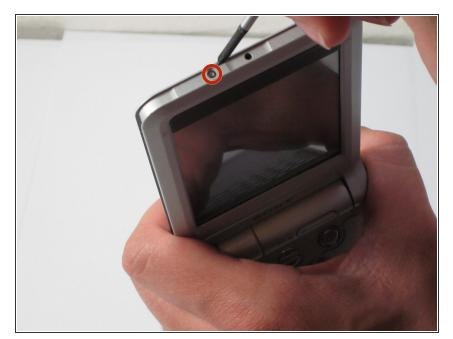
Remove top .75mm screw of the top portion of device with a Phillips #00 screwdriver.
