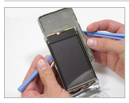
Pry the screen from the back panel using the plastic opening tools to remove the screen module.
