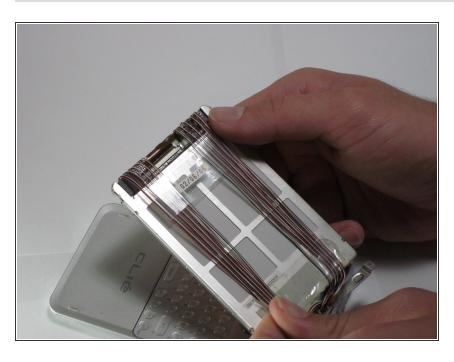
Remove the tape from the wires on the back side of the screen module.
