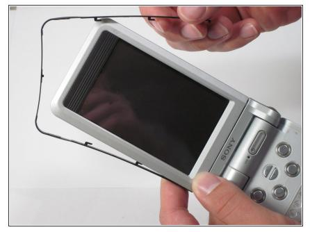
Remove the plastic wrapping on the side of the top portion of the device.
