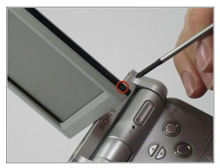
Remove the two 1.5mm screws (one on the right and one on the left side) on the screen portion of the device with a Phillips #00 screwdriver.
