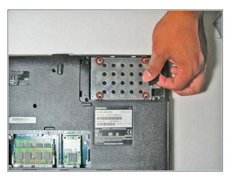
Remove the four 6mm screws with the Phillips #00 screwdriver.
