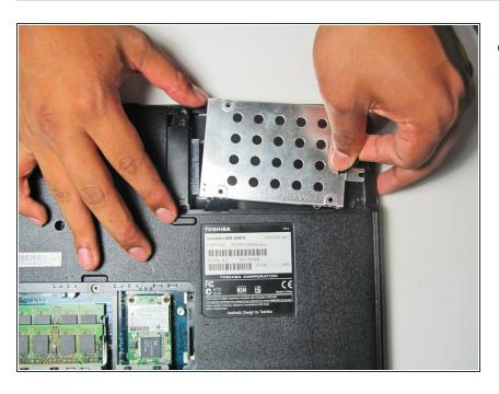
Pull out black tab located on the hard drive to slide it out.
