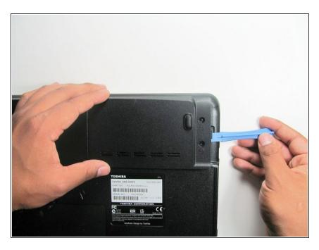
Using a flat head from a plastic opening tool to lift open the cover.
