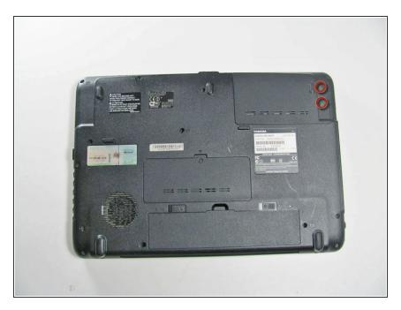
Remove the two 7 mm screws with a Phillips#00 Screwdriver
