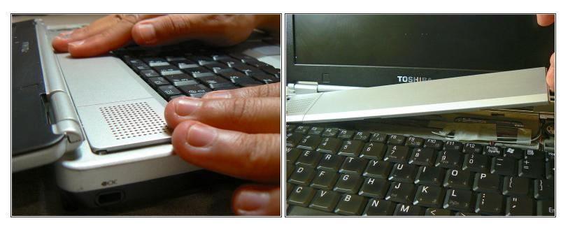
Remove the rest of the cover by sliding it to the right and lifting the edge.
