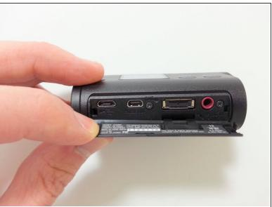
Remove battery. Open bottom hatch. Remove the 2x screws with mini philips driver, the bottom hatch door should just come out with a little pull now.
