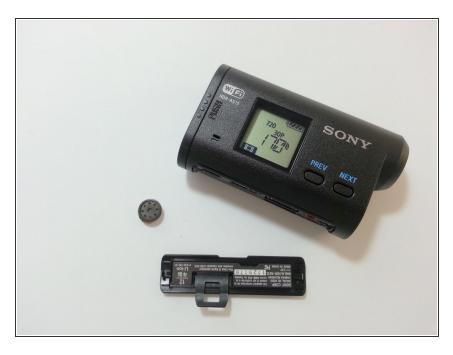
Slide electronics back into the housing. Replace bottom port cover and 2x screws. Replace battery. Cut tether to the bottom hatch, replace on bottom of camera. Enjoy silent operation and hassle-free access to the ports!
