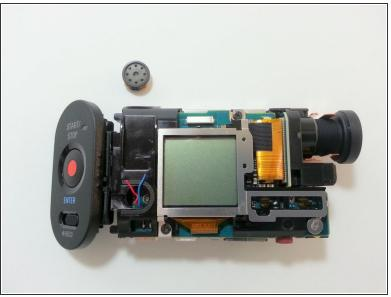
• Remove 2x screws over the metal retaining clip; one is above the LCD and one is below. Gently pull the plastic tab at the top as you swing the metal retaining clip downward. Desolder the speaker. Replace the metal retaining clip and 2x screws.
