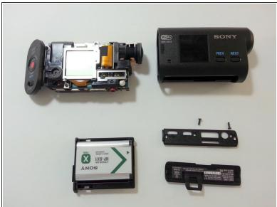
Gently press the tab in the center as you slide out the electronics.
