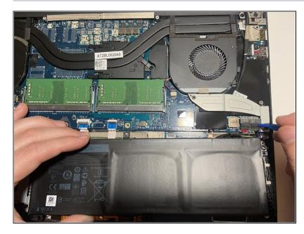
• Use the iFixit opening tool to disconnect the battery connector from the motherboard.
