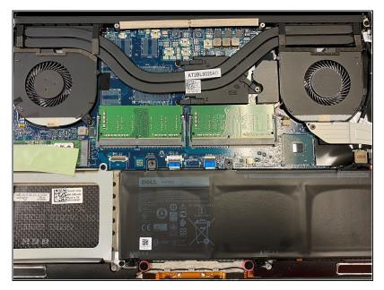
• Lift the back cover off of the device.
