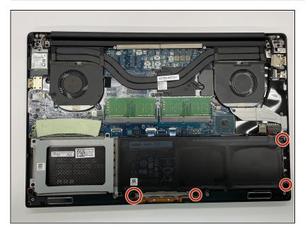
• Using the Phillips #00 screwdriver, remove the four 4 mm screws holding the battery in place.
