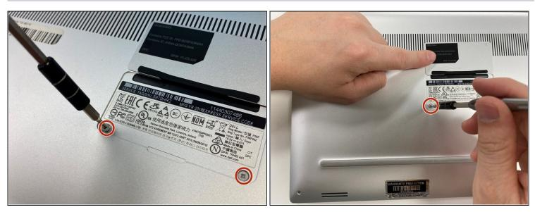
Flip open the system badge and with a Phillips #00 screwdriver, remove the two 8.5 mm screws.
