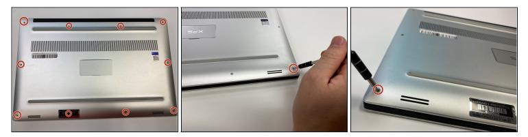
• Using a Torx T5 screwdriver, remove the ten 3 mm screws on the back.
