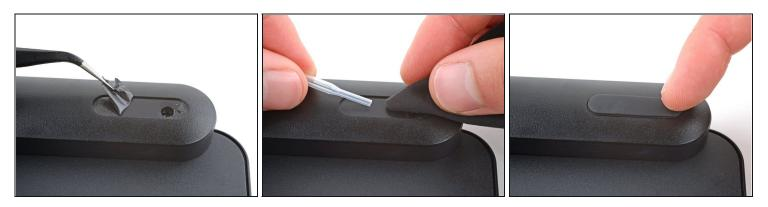
To install a new foot during reassembly:
