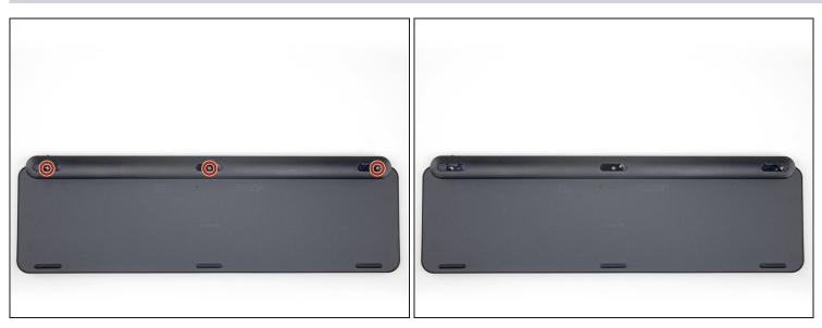
• Use a Phillips screwdriver to remove the three 7.6 mm-long screws securing the battery cover.
