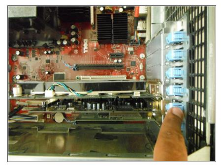
To release the sound card from the motherboard casing: find the blue tab that is the third from the bottom (fifth from the top), and press down and to the right on the tab.
