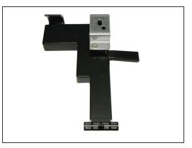
• To remove the support below the processor: press down on the latch at the top of the support, then pull the support outwards, towards yourself.
