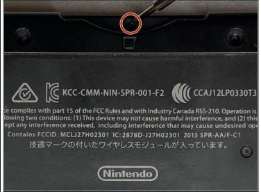
Remove the screw near the game card compartment using a Phillips #00 screwdriver.
