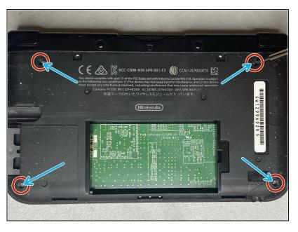
Remove the four screws on the battery panel using the Phillips #00 screwdriver.
