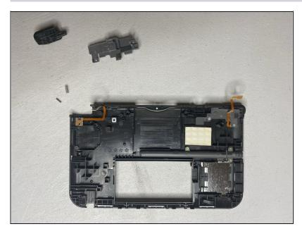
Separate the bumper from the bumper assembly
