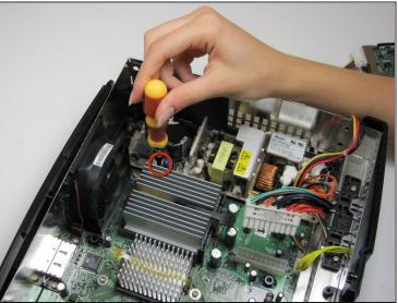
Using T10 Torx screwdriver, remove two 3mm screws from the tan power supply board.
