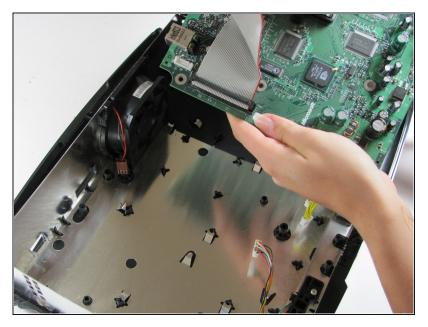
Remove the motherboard from the Xbox. As long as all of the screws are out and the fan is disconnected, it will lift out easily.
