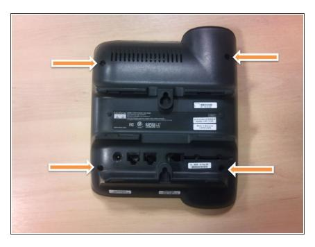
Remove the 4 screws securing the back .
