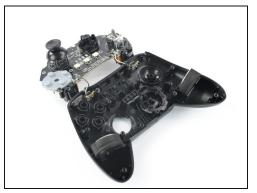
Flip over the mainboard and place it above the controller housing.
