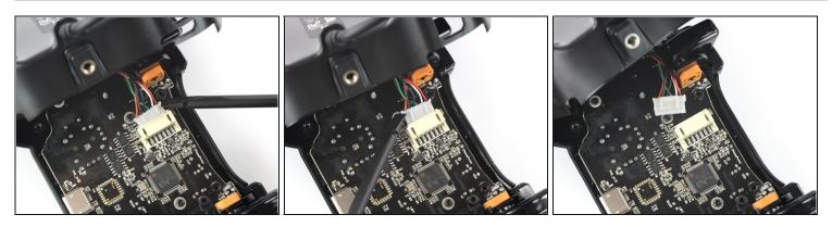
• Use a spudger to disconnect the phone connector cable from the mainboard.
