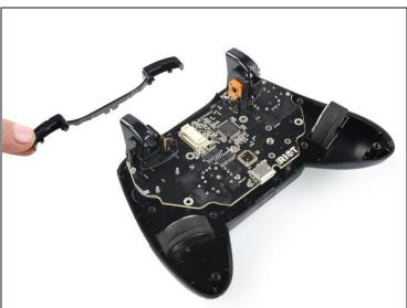
• Remove the shoulder buttons by lifting them out of the case.
