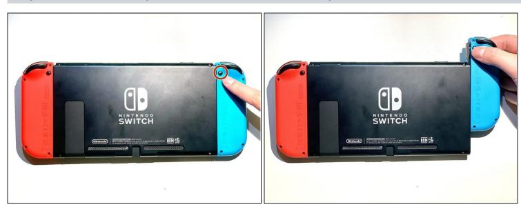
Press and hold the black round button on the back of the Joy-Con, then slide it forward to remove.
