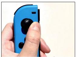
• Rotate the Joy Stick for 30 seconds to allow full penetration of the liquid inside.
