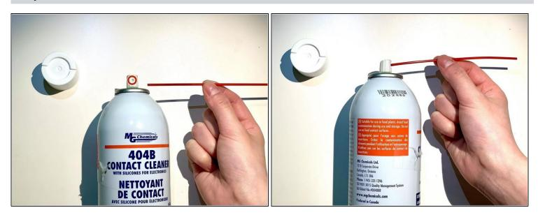
• Open the 404B contact cleaner and insert the tube into the nozzle.
