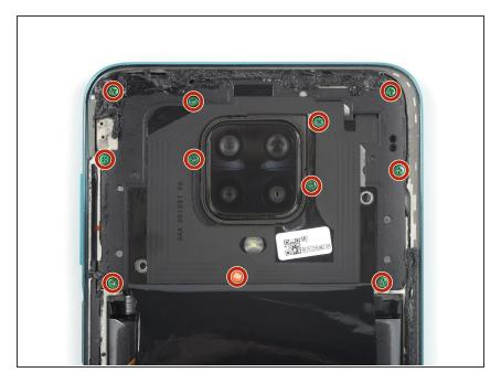
Use a Phillips screwdriver to remove the eleven 3.9 mm-long screws securing the motherboard cover.
