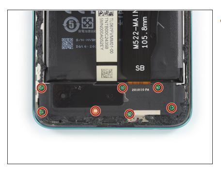
Use a Phillips screwdriver to remove the seven 3.9 mm-long screws securing the loudspeaker assembly.
