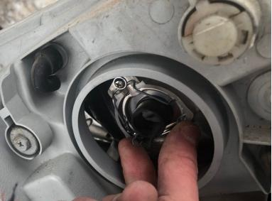
Start the new headlight installation by placing the headlight mount into the headlight housing and secure it with the clip by pinching the ends together and hooking it under the edges of the housing.
