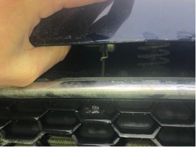
Release the lever under the hood and lift it up to release the hood completely. Simultaneously lift the hood and prop it up with the hood prop securing it in an open position.
