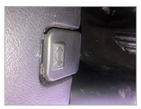
Pull the hood release lever underneath the steering wheel to release hood lock.
