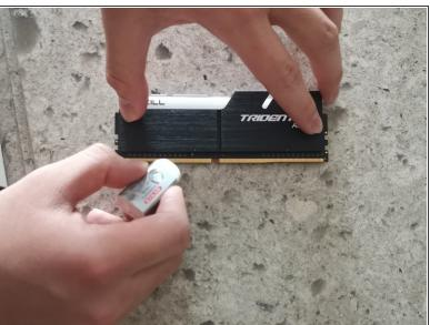
• Use the rubber to clean the connecting finger of the RAM.
