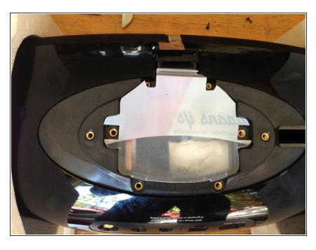
Find something to cover up the hole. This prevents the glue from sticking to internal parts. I used the cover of a plastic ice box.
