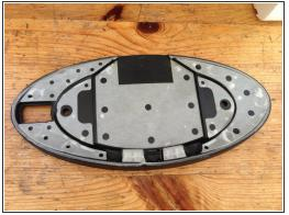
Remove the rubber on the bottom. Slowly pull it up from one side. It's attached with glue.
