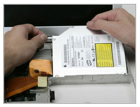
Free the inverter cable and Airport antenna cable from the corner of the optical drive and lift the drive up so that it stands vertical.
