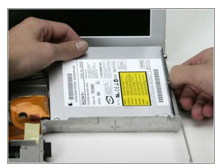
Pull out on the right edge of the metal casing and lift the edge of the optical drive up.
