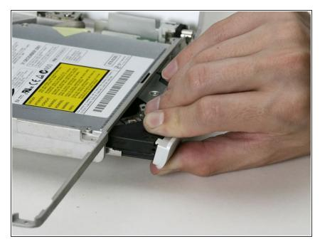
Pry up the white plastic tab on the other end of the drive. Pull the optical drive faceplate off, rotating it up and down slightly to get over the remaining two tabs.
