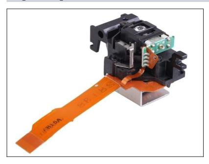
Once the laser lens is carefully separated from the optical drive assembly, insert the new laser into the optical drive assembly and follow these steps in reverse order for reassembly.
