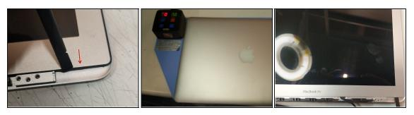
Remove the gasket that runs along the perimeter of the display. You can use a spudger to pry up the bezel and tweezers to pull it
