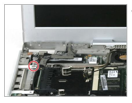
Remove the single Phillips from the white plastic finger of the IO Bezel.
