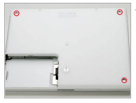
Remove the three newly-revealed Phillips screws.
