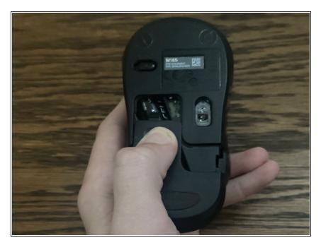
Remove back cover by pressing down carefully on the creased part, then pull down.
