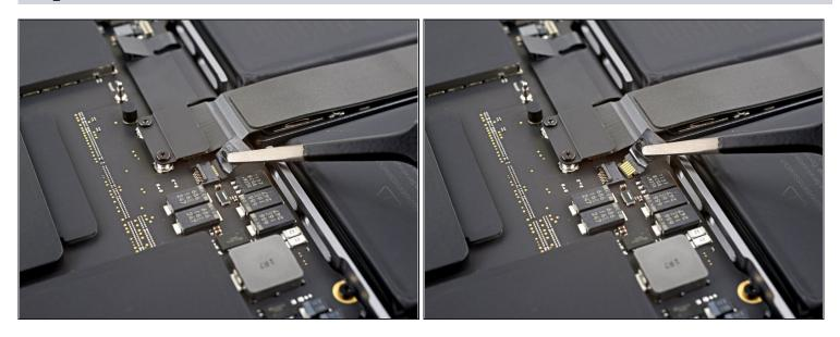
Disconnect the battery board data cable by sliding it out from its socket on the logic board.
