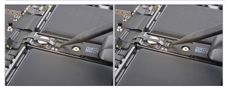
• Use a spudger to gently pry up the locking flap on the ZIF connector for the battery board data cable.
