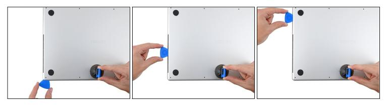
Repeat the previous step on the other side, using an opening pick to to release the second clip.
