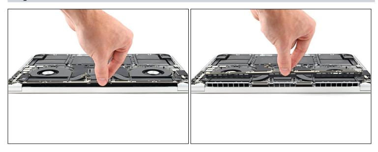
• Pull the antenna bar straight up and out of the frame to remove it.
