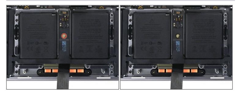
• Use a T5 Torx driver to remove the 4 mm 5IP Torx Plus screw securing the battery board.
