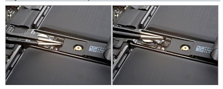
• Peel back any tape covering the battery board data cable connector under the large pancake screw.
