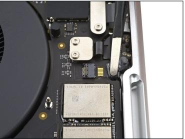
• Disconnect the microphone cable by sliding it out from its socket on the logic board.
