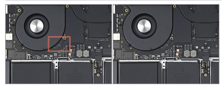
• Repeat the previous disconnection and reposition procedure for the left fan.
