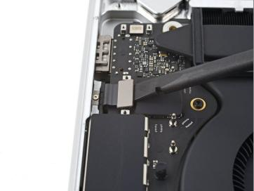
Use a spudger to pry up and disconnect the left USB-C port's press connector.
