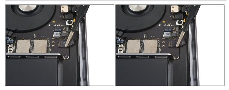
• Disconnect the right speaker cable by sliding it out from its socket on the logic board.
