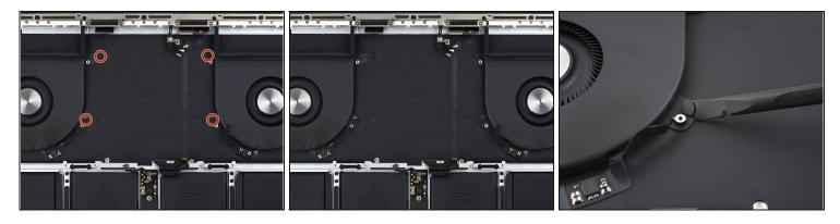
Use a spudger to remove the four screw covers.
