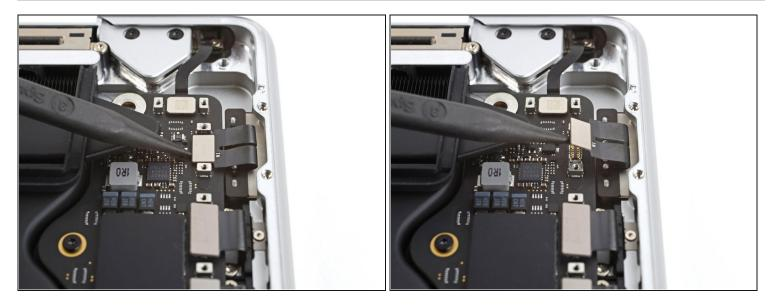
Use a spudger to pry up and disconnect the MagSafe port's press connector.
