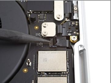
• Use a spudger to gently pry up the locking flap on the ZIF connector for the microphone cable.
