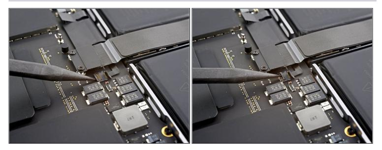
• Use a spudger to gently pry up the locking flap on the <u>ZIF connector</u> for the battery board data cable.
