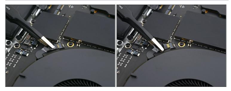
• Disconnect the right fan cable by sliding it out from its socket on the logic board.
