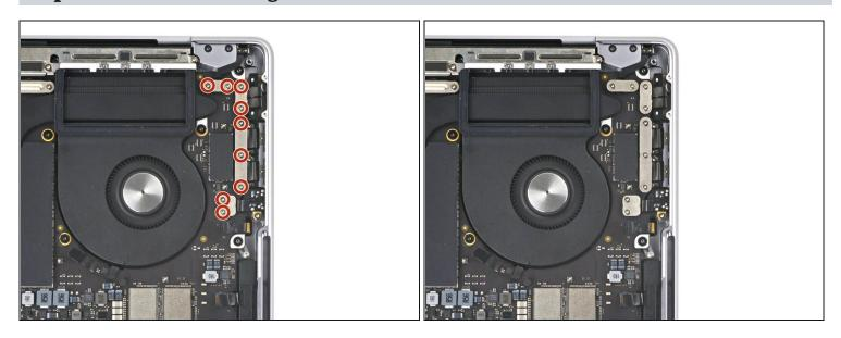
• Use a T3 Torx driver to remove the nine 2.1 mm screws securing the right cable covers to the frame:
