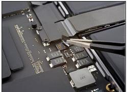
• Peel back any tape covering the battery board data cable connector on the logic board.
