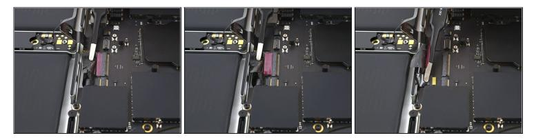
Disconnect the keyboard and keyboard backlight cables by sliding them out from their sockets on the logic board.
