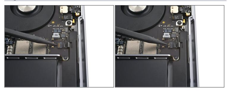
• Use a spudger to gently pry up the locking flap on the ZIF connector for the right speaker cable.
