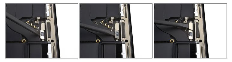
• Use the flat end of a spudger to pry up and disconnect the right-most screen cable press connectors secured to the logic board.
