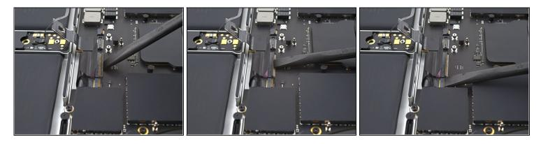
• Use a spudger to gently pry up the locking flap on the ZIF connectors for the keyboard cables.
