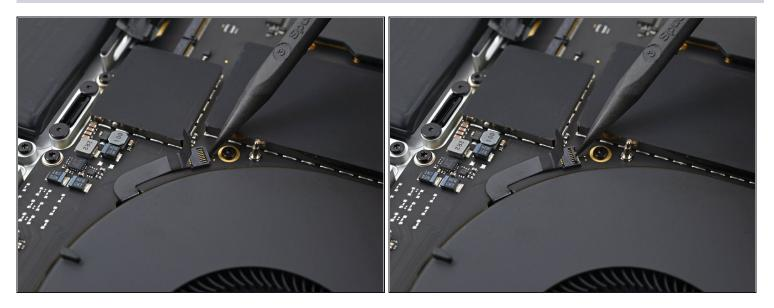
• Use a spudger to gently pry up the locking flap on the ZIF connector for the right fan cable.
