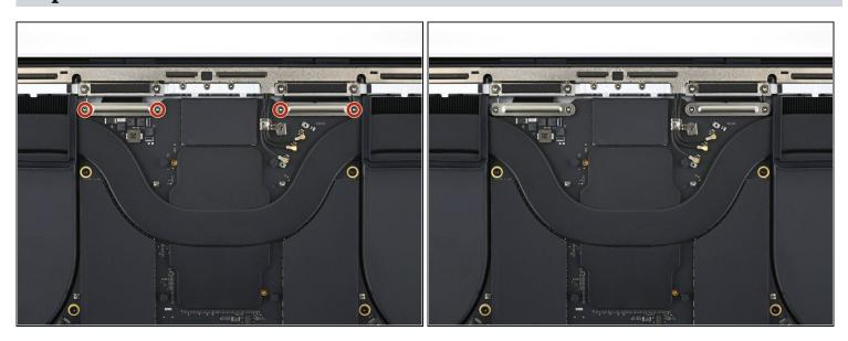
• Use a T3 Torx driver to remove the four 2.1 mm screws securing the screen cable covers.
