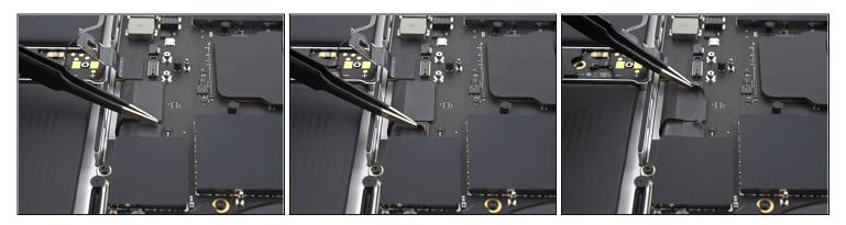
• Peel back any tape covering the <u>keyboard and keyboard backlight cable connectors</u>.
