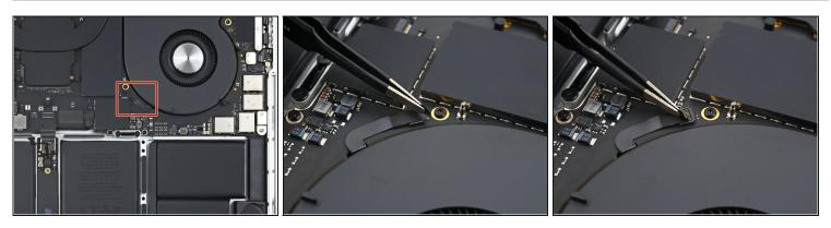
• Peel back any tape covering the right fan cable connector.
