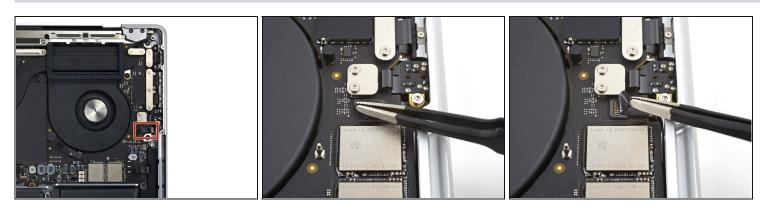
• Peel back any tape covering the microphone cable connector.
