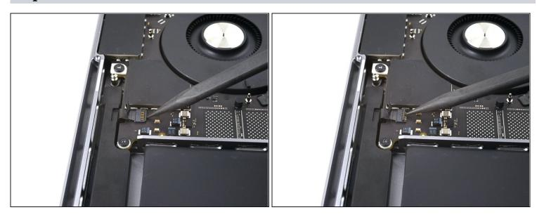
• Use a spudger to gently pry up the locking flap on the ZIF connector for the left speaker cable.
