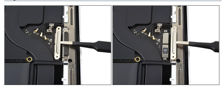
Use tweezers, or your fingers, to remove the two screen cable covers from the logic board.
