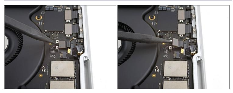
• Use a spudger to pry up and disconnect the headphone jack's press connector.
