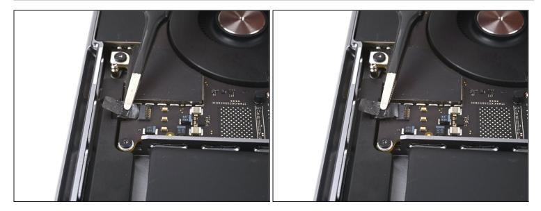
• Disconnect the left speaker cable by sliding it out from its socket on the logic board.
