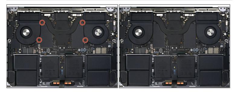
• Remove the four black screw covers from the logic board.
