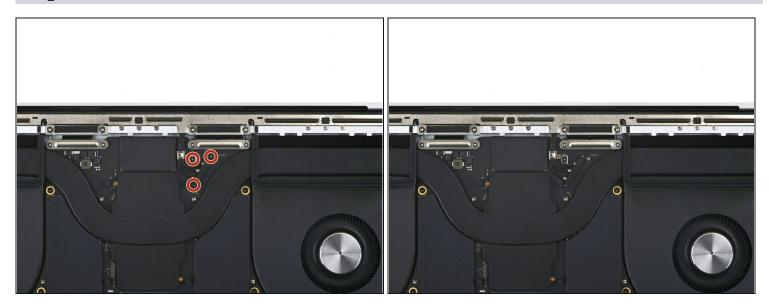
• Use a T3 Torx screwdriver to remove the three 2.1 mm screws securing the antenna board bracket and coaxial cable cover to the frame.
