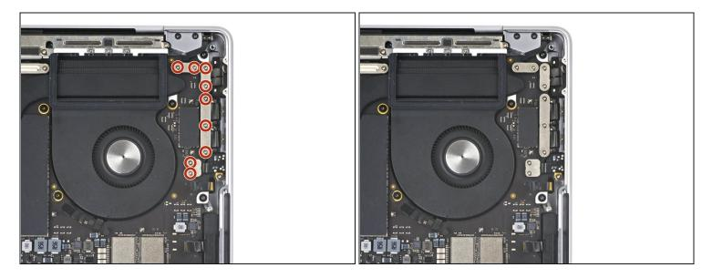
• Use a T3 Torx driver to remove the nine 2.1 mm screws securing the right cable covers to the frame:
