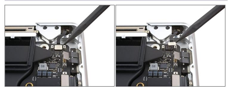
• Use a spudger to pry up and disconnect the lid angle sensor's press connector.
