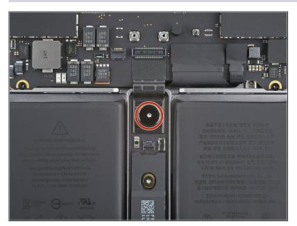
Use a T5 Torx driver to remove the 3.8 mm 5IP Torx Plus widehead screw securing the battery power connector.
