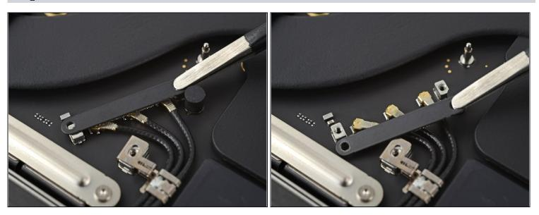
• Use tweezers, or your fingers, to remove the cover on top of the antenna bar's coaxial cables.
