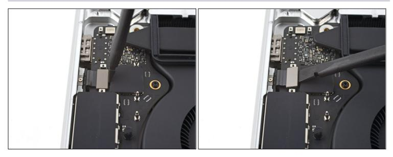
• Use a spudger to pry up and disconnect the left USB-C port's press connector.
