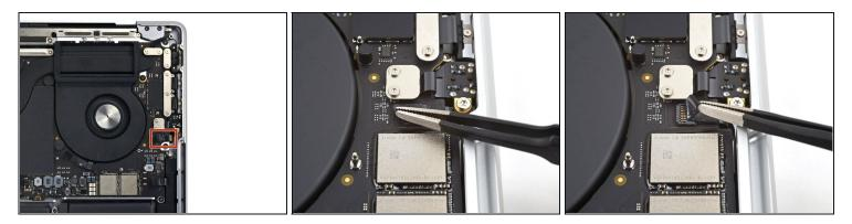
• Peel back any tape covering the microphone cable connector.
