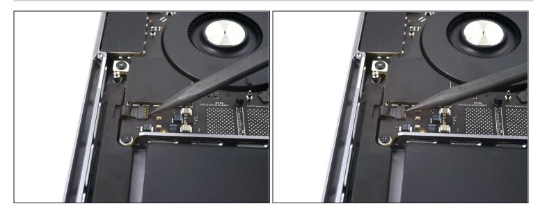
• Use a spudger to gently pry up the locking flap on the ZIF connector for the left speaker cable.
