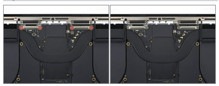
• Use a T3 Torx driver to remove the four 2.1 mm screws securing the screen cable covers.
