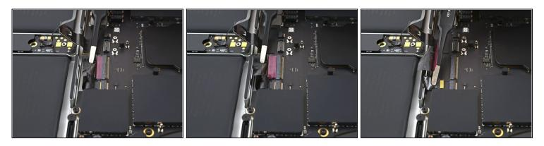
• Disconnect the keyboard and keyboard backlight cables by sliding them out from their sockets on the logic board.
