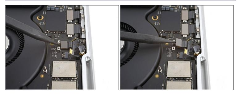
• Use a spudger to pry up and disconnect the headphone jack's press connector.
