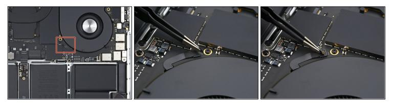
• Peel back any tape covering the right fan cable connector.
