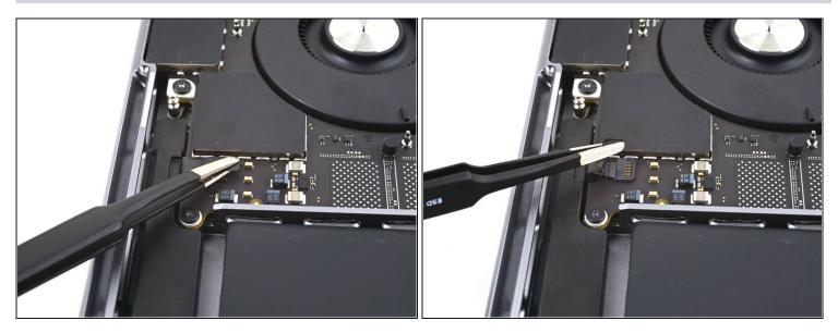
• Peel back any tape covering the left speaker cable.
