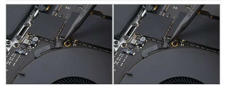
• Use a spudger to gently pry up the locking flap on the ZIF connector for the right fan cable.
