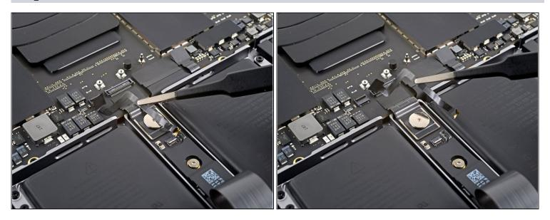
(*i*) The battery board data cable is lightly adhered to the device.
