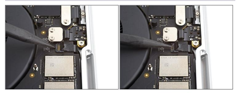
• Use a spudger to gently pry up the locking flap on the ZIF connector for the microphone cable.
