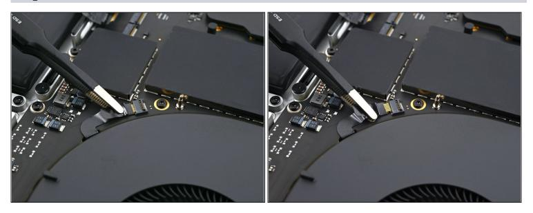
• Disconnect the right fan cable by sliding it out from its socket on the logic board.
