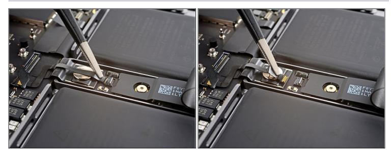
• Disconnect the battery board data cable by sliding it out from its socket on the battery board.
