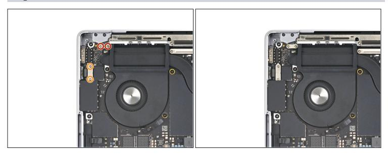
• Use a T3 Torx driver to remove the four screws securing the left cable covers to the frame:
