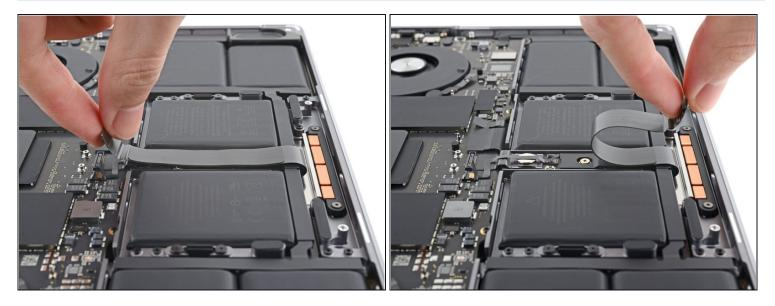
(*i*) The trackpad cable is lightly adhered to the frame.
