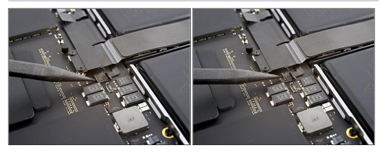
• Use a spudger to gently pry up the locking flap on the <u>ZIF connector</u> for the battery board data cable.
