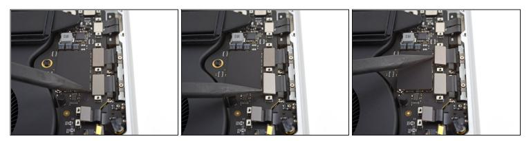
• Use a spudger to pry up and disconnect the right USB-C ports' press connectors.
