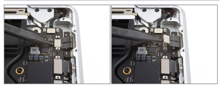
• Use a spudger to pry up and disconnect the MagSafe port's press connector.
