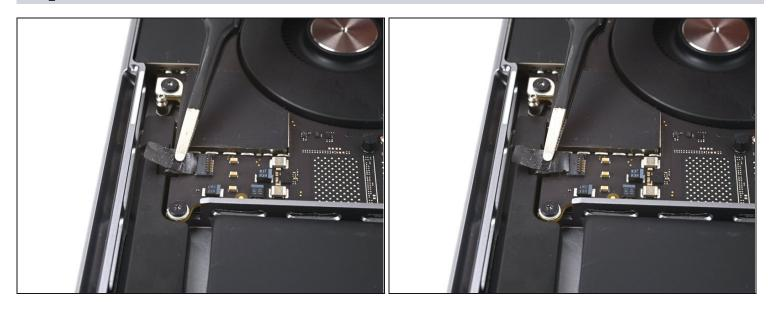
• Disconnect the left speaker cable by sliding it out from its socket on the logic board.
