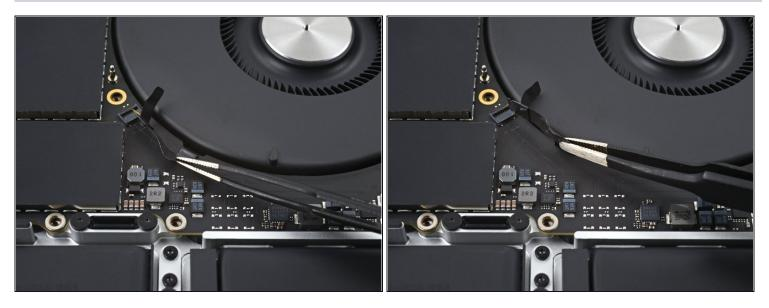
(i) The right fan cable is lightly adhered to the logic board.
