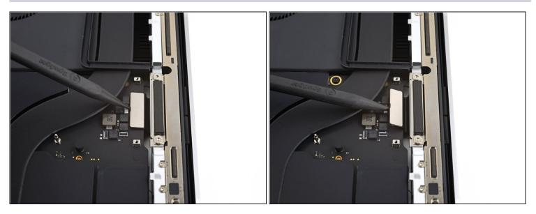
• Repeat the previous disconnection process for the remaining press connector at the top left of the logic board.
