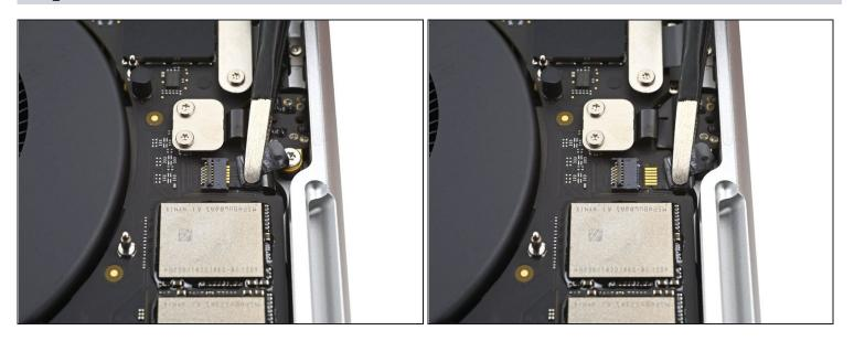
• Disconnect the microphone cable by sliding it out from its socket on the logic board.
