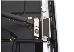
• Use the flat end of a spudger to pry up and disconnect the two right-most screen cable press connectors secured to the logic board.
