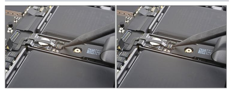
Use a spudger to gently pry up the locking flap on the ZIF connector for the battery board data cable.
