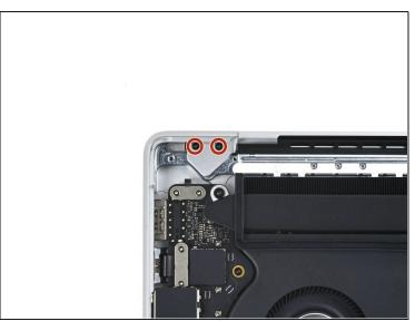
• Use your T5 Torx driver to remove the two 2.5 mm-long 5IP Torx Plus screws securing each hinge cover (four screws in total).
