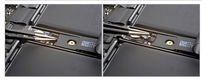
Peel back any tape covering the battery board data cable connector under the large pancake screw.
