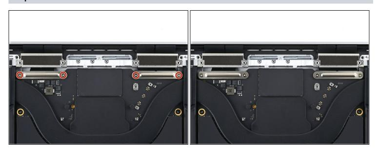
Use a T3 Torx driver to remove the four 2.1 mm 3IP Torx Plus screws securing the screen cable covers.
