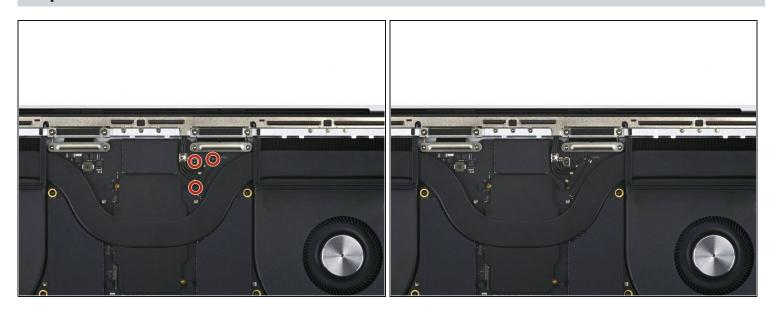
• Use your T3 Torx driver to remove the three 2.1 mm-long 3IP Torx Plus screws securing the antenna connector cover and bracket.
