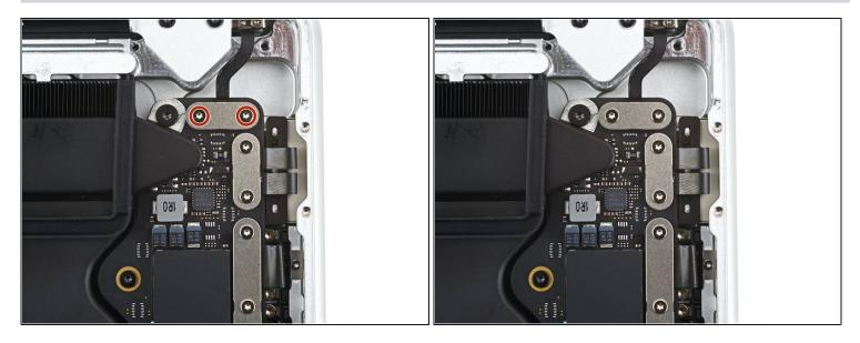
Use a T3 Torx driver to remove the two 2.1 mm 3IP Torx Plus screws securing the lid angle sensor cover near the right hinge.
