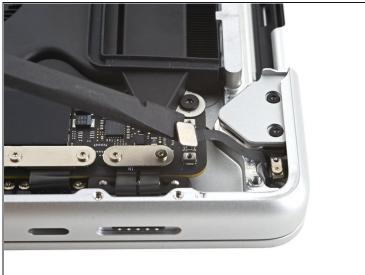
Use the flat of a spudger to pry up and disconnect the lid angle sensor's press connector.
