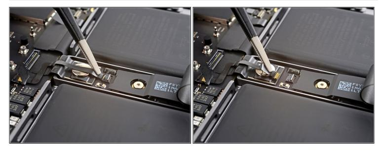
• Disconnect the battery board data cable by sliding it out from its socket on the battery board.
