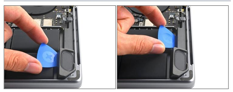
• Slide the pick along the edge of the speaker to separate the adhesive.
