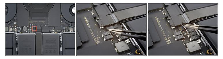
• Peel back any tape covering the battery board data cable connector on the logic board.
