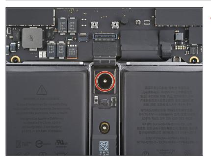
Use a T5 Torx driver to remove the 3.8 mm 5IP Torx Plus widehead screw securing the battery power connector.
