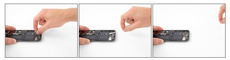
• Repeat the previous step to remove the strip on the opposite side, leaving the center strip for last.
