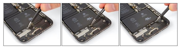
• Repeat the above step to separate the remaining two adhesive tabs from the bottom edge of the battery.
