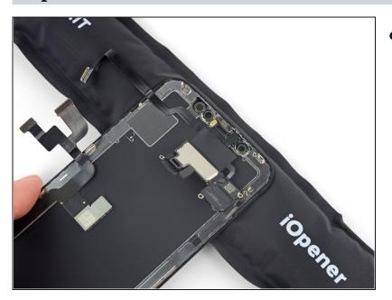
• Use a hairdryer or heat gun or prepare an iOpener and apply it to the top front of the display for about a minute, in order to soften the adhesive securing the sensors.
