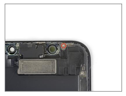
Remove the 1.2 mm Y000 screw on the back of the display assembly, near the infrared camera port.
