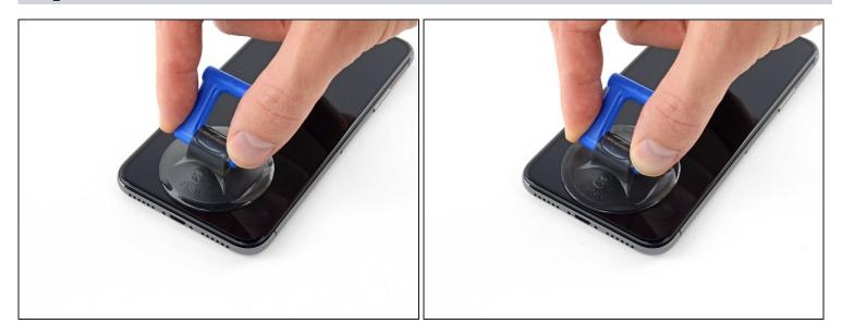
• If using a single suction handle, apply it to the bottom edge of the phone, while avoiding the curved portion of the glass.
