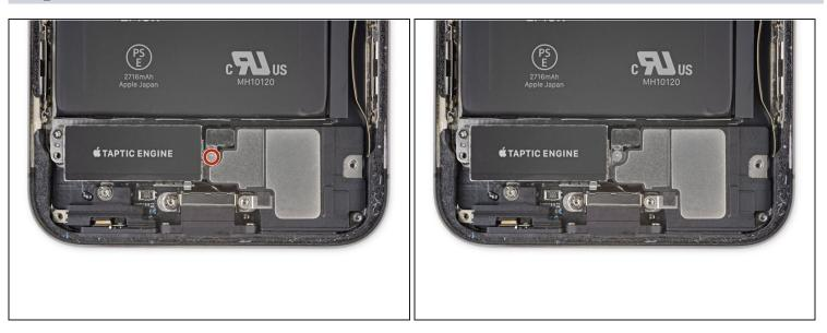
• Remove the 2.1 mm Y000 screw securing the speaker connector cover.
