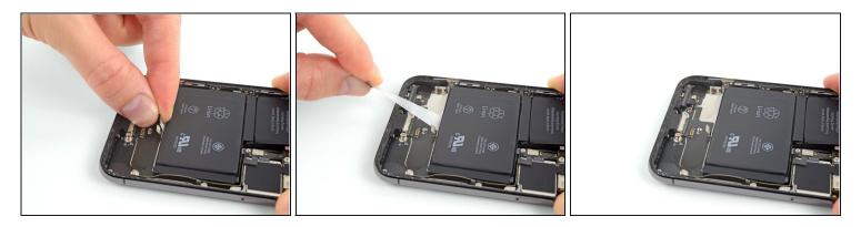
• Remove the center strip, being careful not to snag it on the speaker flex cable.
