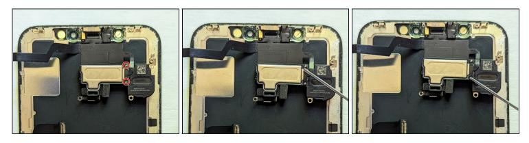
Apply flux to the two solder points.
