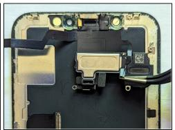
Remove the tape covering the solder points.
