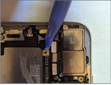
• Disconnect the WiFi Antenna cable connector.
