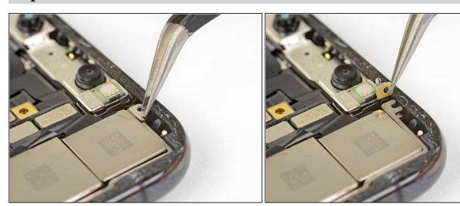
• Use <u>tweezers</u> to gently fold the small metal grounding bracket out of the way. Do not pull up on it as it is connected to a fragile flex cable.
