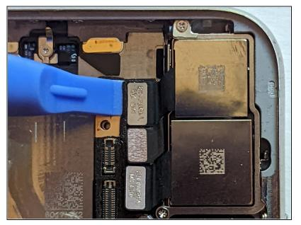
• Disconnect the Wide-Angle Camera cable connector.
