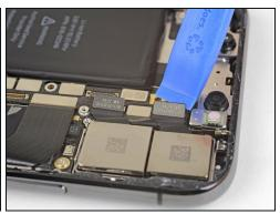
Use an opening tool or fingernail to disconnect the two camera connectors by prying them straight up from their sockets.
