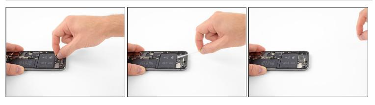
Repeat the previous step to remove the strip on the opposite side, leaving the center strip for last.
