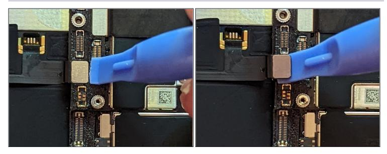
• Disconnect the Button / Wireless Charging cable connector.
