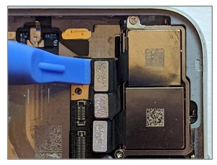
• Disconnect the Wide-Angle Camera cable connector.
