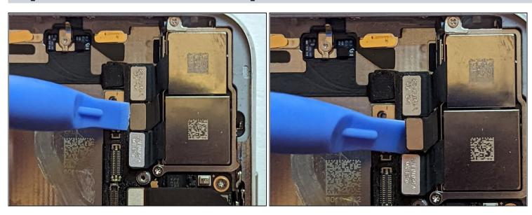
• Disconnect the Power Button / Flash / Microphone cable connector.
