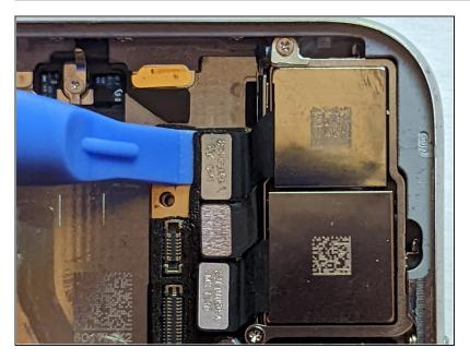
Disconnect the Wide-Angle Camera cable connector.
