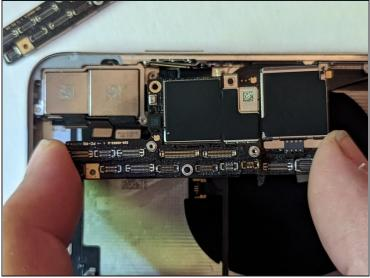
• The logic board assembly is mounted on two posts going through the lower board and are secured to the upper board. In order to remove it, you must lift it evenly straight up to clear the stand-offs.
