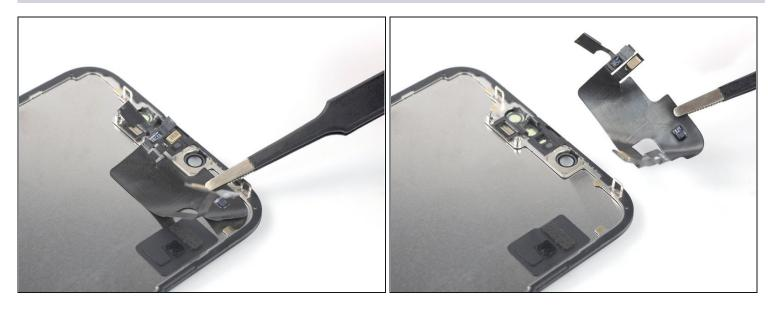
• Remove the front sensor assembly.
