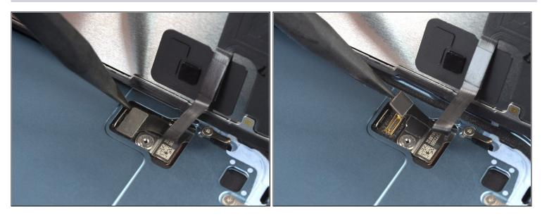
• Use the pointed end of a spudger to disconnect the front sensor cable by prying the connector straight up from its socket.
