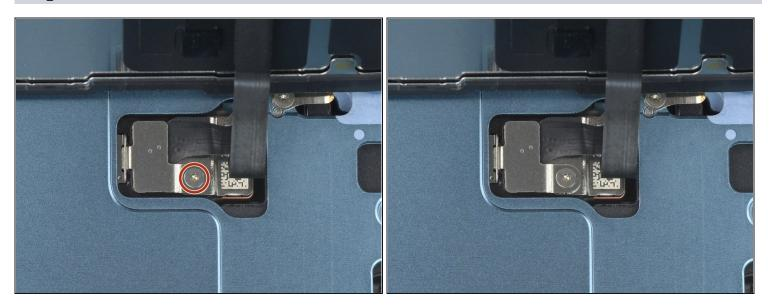
Use a Y000 screwdriver to remove the 0.9 mm-long screw securing the front sensor connector bracket.
