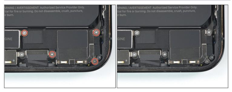
• Use a Phillips driver to remove the four 1.5 mm-long screws securing the loudspeaker.
