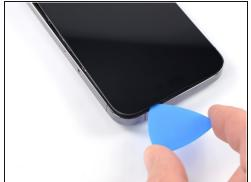
• Insert your pick underneath the top right edge of the phone. Slide it around the topright corner and half way across the top edge stopping right before the earpiece speaker cut-out.
